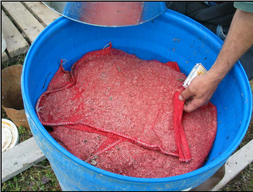
Photo #18. Petroleum absorbent material in a scrubber barrel.
