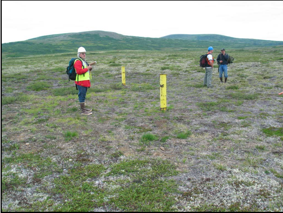
Photo #9. Piezometer wells P4A.
