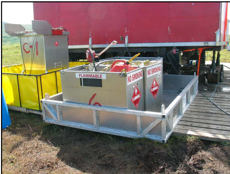
Photo #17. Double walled, 118 Gal. fuel transport tanks in aluminum containment.
