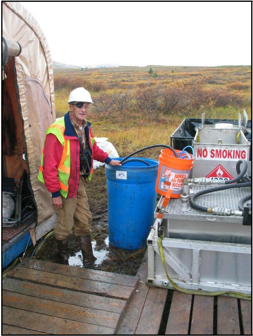
Photo #3. Gary Martello processing water from a containment berm through a scrubber barrel to remove any petroleum products. All containment berms are cleaned by this process as needed after rains.
