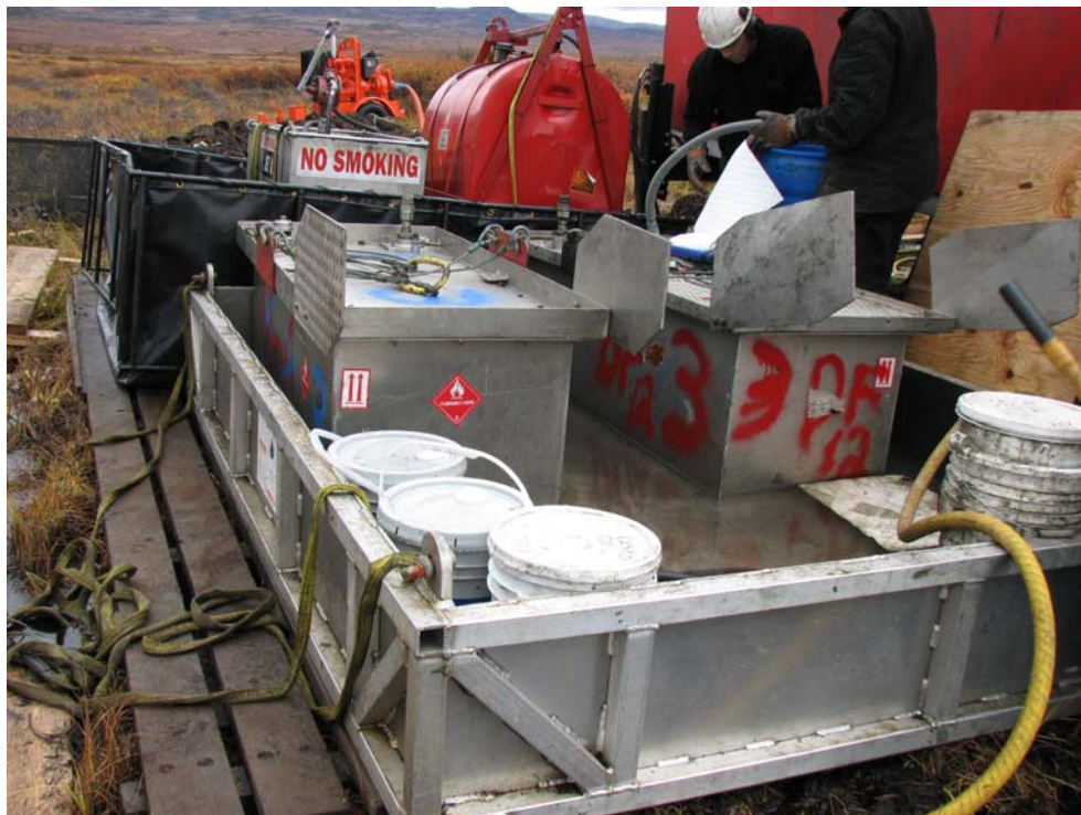
Photograph No. 7: Drill Site No 7385 Note standing water in secondary fuel catchment basin.
