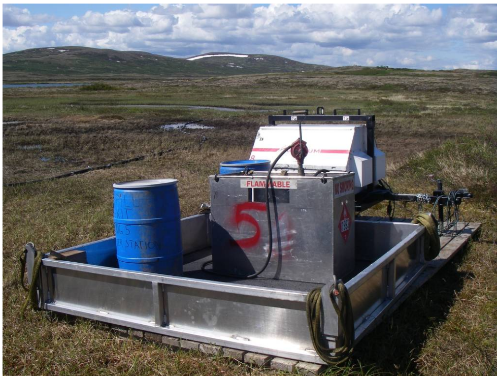
Figure 4. Fuel containment area, drill rig 8407 (No. 5).
