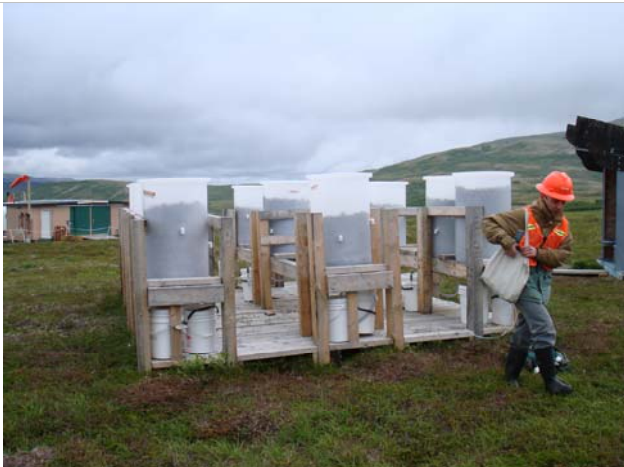
Figure 9. Long-term geochemical barrel tests.
