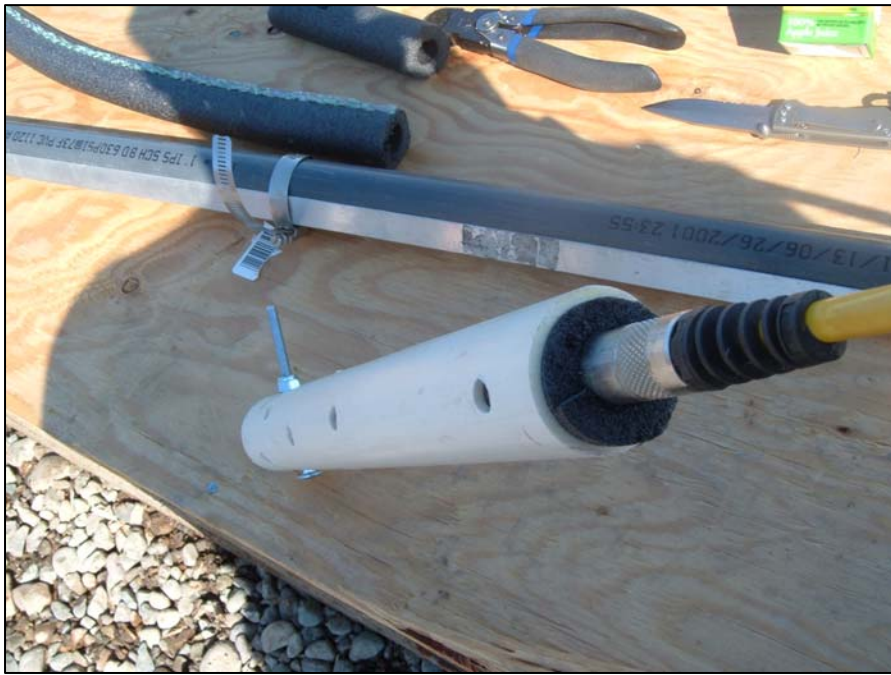
PHOTO 4.1-1: Close-up of datalogger/transducer fixed in stilling-well
