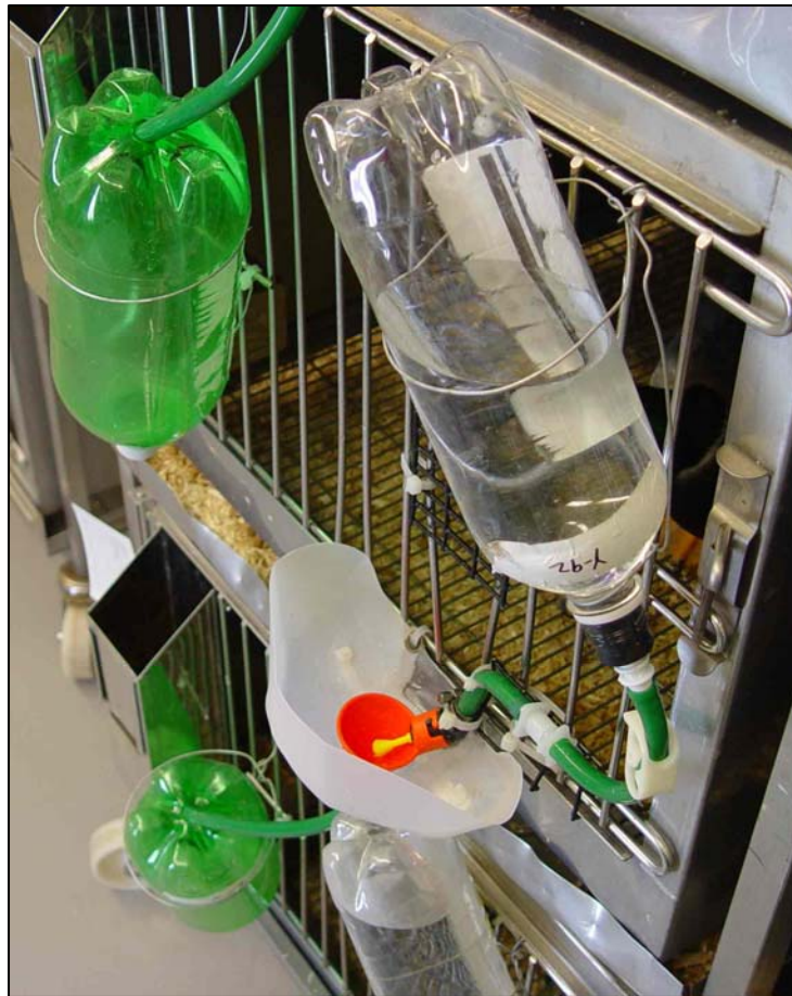
Figure 2. Water provision and waste collection system – view from above. Ducks press the yellow bar in the sipper cup, which releases drinking water into the cup. Some ducks play with the sipper cups, resulting in increased waste water. Waste collection system allows quantification of waste spillage, avoiding incorrect interpretation of drinking rates.
