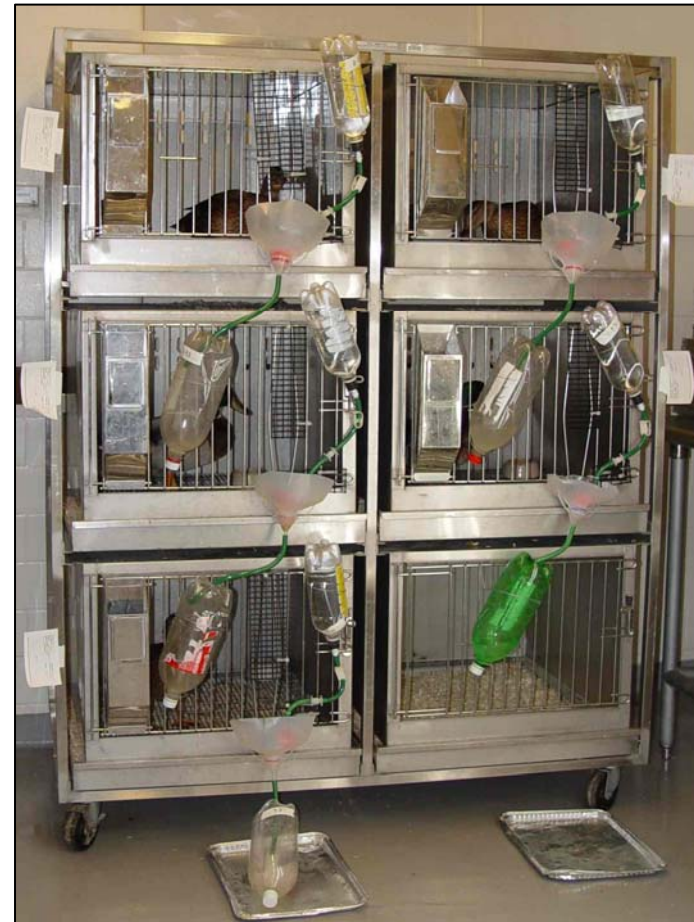
Figure 3. Mallard ducks are maintained in stainless steel rabbit cages modified for collection of water consumption and spillage data. Consistent lighting for each cage is maintained using fluorescent lamps mounted vertically adjacent to the cage rack
