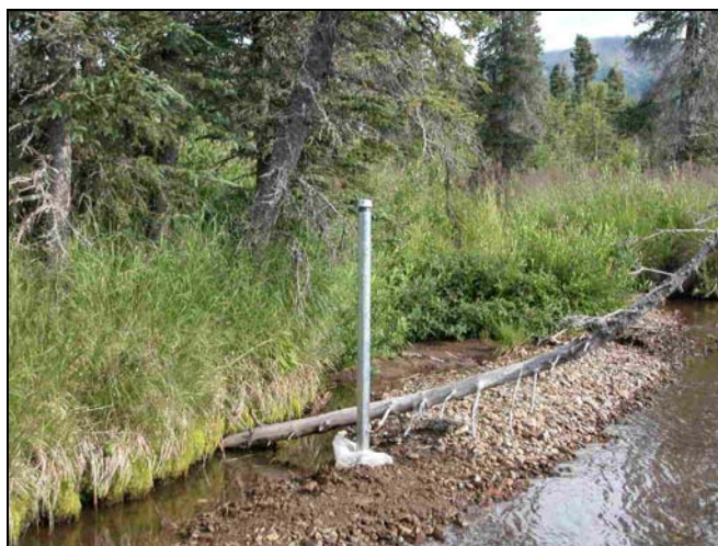
FIGURE 4-26. Example of newly installed crest gauge
